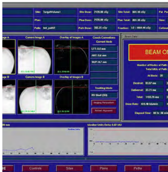
Fig. 3: Screenshot of the CyberKnife control software. On the left are digitally reconstructed X-ray images computed from CT images. In the middle are intra-operative X-ray images on which the digitally reconstructed images are superimposed on the right in order to check the tumour localisation visually. From: http://en.wikipedia.org/wiki/File:6DSkull.jpg , © 2007 Wikipedia User Steven3045 (last accessed at 11 am on 20/02/2014)
