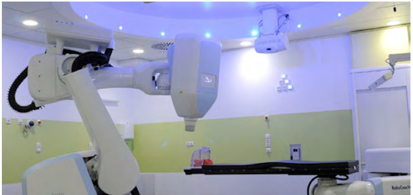
Fig. 1: Technical arrangement of US manufacturer Accuray's CyberKnife radiosurgery system used on the Berlin Charité's Virchow campus. On the left the robot arm with the linear accelerator head and on the right the RoboCouch for patients, with a thermoplastic mask screwed into place.
